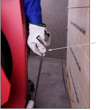
...but about 10cm below the strap lifter. Hold the strap with the whole hand and pull it out of the strapping system. At the same time, you have to let the end of the strap slide through your other hand!
