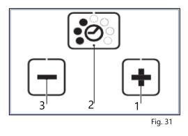
– Save: Press "welding time" button (2) or wait for 5 seconds.
