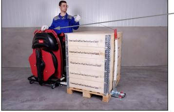
... move the ChainLance completely back by pushing the joystick in "move in" direction.
