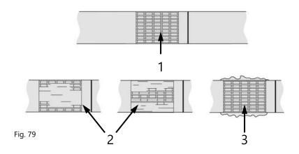
**1 Good welding:** The whole sealed surface has been properly welded without any extra material being squeezed out to the side.
